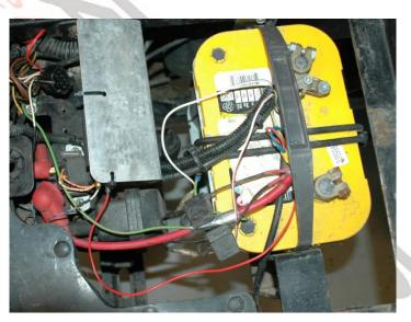
Now the ignition unit must be connected to switched 12V. Under the bonnet next to the horn you will find 2 connectors. One of these connectors has a red/white wire. You must attach the red wire provided in this conversion kit to the red/white (original) wire. You can do this by using the blue attachment as shown in the picture below. Place the new red wire parallel next to the other wires. You can remove the section under the pedals for better access.
