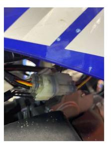
Plug the supplied wiring loom between the connectors of the ignition lock.
