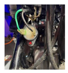
Securely tape the black wire to the wiring loom. It needs to stay unconnected.
