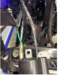
Screw the ignition coil to the same location as the old one with the M5 bolt and spacer. Use the
